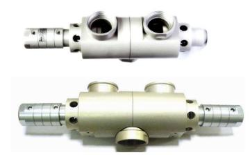
The valve performs as a double of vacuum / vacuum-breaker valve having a central common pipe connection and is pneumatically actuated by a double-acting cylinder; it has therefore 2 flat shutters, 3 pipe connections 2" and 2 exhaust ports. when one exhaust port is closed the other is open and vice-versa.
