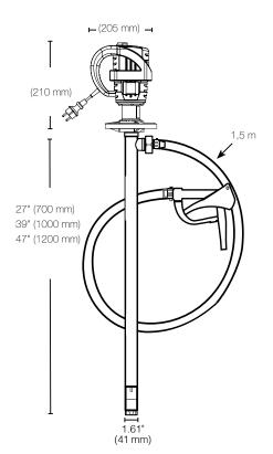
Engineered for transferring corrosive chemicals associated with the water treatment industry. Robust Polypropylene offers excellent durability and chemical resistance against light to aggressive chemicals.
