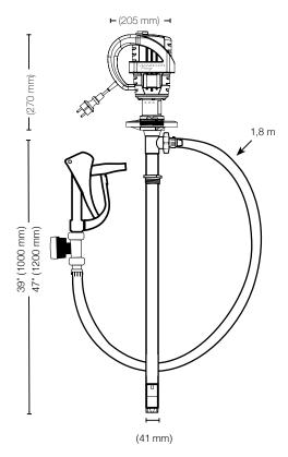
Engineered for transferring highly concentrated and aggressive liquids. Robust PVDF ensures excellent durability and chemical resistance against light to aggressive chemicals. Equipped with a battery powered turbine flow meter for controlling, measuring and dispensing neutral liquids, corrosive chemicals (acids & alkalis) and many other non-flammable liquids.
