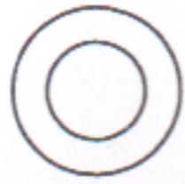
96292 (8) "O" RING (2.5 mm X 12mm O.D.) "FOR NON-METALLIC CENTER SECTION"
