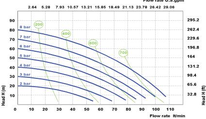
\* The curves and performance values refer to pumps with submerged suction and a free delivery outlet with water at 20°C, and vary according to the construction material.
