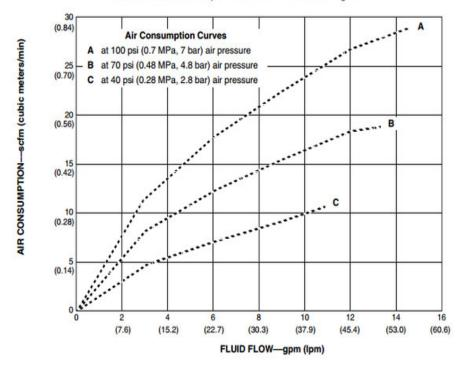
To find Pump Air Consumption (scfm or m³/min) at a specific fluid flow (gpm/lpm) and air pressure (psi/MPa/bar):
