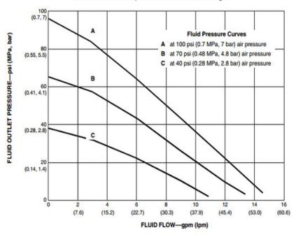
To find Fluid Outlet Pressure (psi/MPa/bar) at a specific fluid flow (gpm/lpm) and operating air pressure (psi/MPa/bar):
