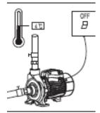
In case ambient temperature is lower than 4°C or the pump is not used for a long time, empty liquid the pipeline system to avoid ice cracking of the pump chamber.
