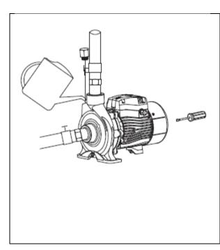
Rotate the fan blade before start- up, check whether the pump rotation is flexible and then unscrew the water-filling plug, fill the pump chamber with clean water from the water injection hole, then tighten the plug screw after the air has been completely discharged. The valve should be shut tightly while starting up the pump. After the pump discharges water operates normally, adjust the valve to the required flow (working range is displayed on the nameplate).
