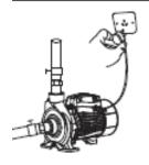
Ensure the pump will not be accidently turned on while installing and maintaining; if not used for a long time, cut off the power first and then turn off valves in inlet and outlet of the pump.
