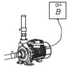
The pumped liquid maybe hot and under high pressure, before moving and demounting the bump, valves in both sides of the bump should be turned off first and then empty liquids in the pump and pipelines so as not to be scalded.
