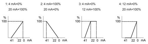
Examples 3 and 4 can be combined into two pumps when both are controlled with the same mA signal to start a second pump as supplementary flow.
