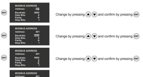
Address: 001 (ENT Baudrate: 9600 Data Bits: Stop Bits:
