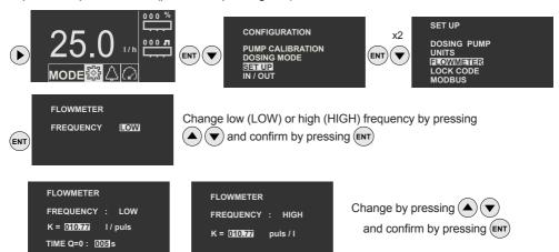
TIME Q=0, Time interval (seconds) between two pulses to consider zero flow.
