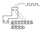
The pulse output isolator allows any device to be securely connected to a pulse output.
