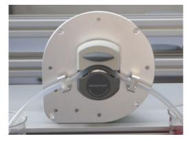
④Fix the tube clamp at one end of the tube to the left tube clamp, lightly tighten the tube, and fix the other end to the right tube clamp.
