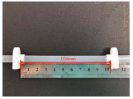
③The two ends of the tube pass through the tube clamps respectively, leaving a length of 104mm in the middle.
