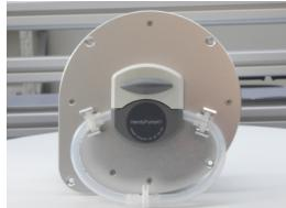
(5) Turn the knob 180 ° clockwise to press the pressure block in place and compress the tube.
