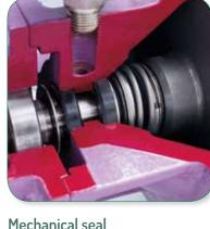
with stainless steel shaft sleeve and lubrication behind the seal to increase the dry running capabilities.
