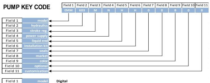
**EMM** Digital constant dosing with manual adjustment, and proportional dosing to an analog input signal (4÷20 mA). Prepared for level probe.
