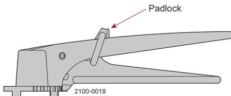
**Figure 1. Lockable Multiposition Handle with padlock**
